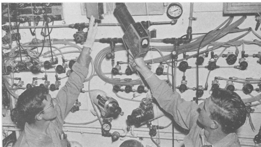
CHECKING RADIATION —Fission product materials emitting high levels of radiation are processed inside a thick walled concrete cell. This shows apparatus on the outside wall where all operations are performed by remote control. Radiation emitted through an opening is being checked with an instrument called a "cutie pie."
