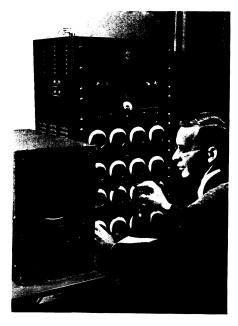
SAVES TIME—A new electronic computing device known as the Antennalyzer, developed at RCA Laboratories, solves the problems of locating and arranging new antennas in a matter of minutes compared to weeks of surveys and calculations heretofore necessary. Readings taken from the final dial settings tell engineers where to locate the antenna towers in order to direct maximum power in desired directions.
