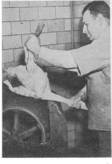
PLUCKING machine removes feathers, even pinfeathers, from fowl at a rate of 200 chickens an hour. Essential parts of the machine are scores of rubber fingers mounted on a drum which turns at high speed. The picture shows a turkey being made ready for market.
