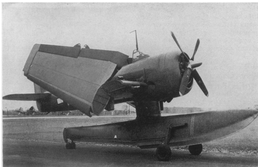
SPACE SAVER —Folding wings are a new feature for a Navy scout-observation seaplane. Shown here on its beaching gear, the new Curtiss Seahawk occupies less space aboard its ship. Official U. S. Navy photographs.
