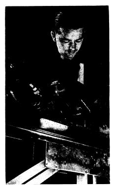
SEWING STEEL — Electric stitches are being made in this stainless steel structure by fusing sheets of metal together wherever the worker applies the electrodes. Resulting connections are much stronger than would be rivets of the same size.
