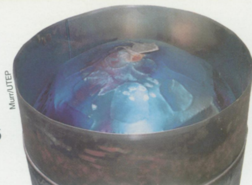
A steelpan held upside-down over a fire turns blue from oxidization. Heat ages the steel, modifying the drum's sound.
