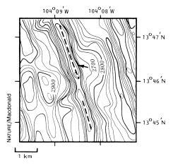
In this depth-contour picture of part of the East Pacific Rise, the ridge axis (dotted line) is interrupted by a SNOO. Batiza and Margolis interpret the region to the southwest of the axis, in which the contour lines veer sharply away from the ridge, as a fault that grew perpendicular to the ridge during the spreading process.
