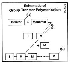
In the new method of making polymers, small molecules, called monomers (M), insert between an initiator (I) and its activating group (G), so that the activating group repeatedly is transferred to the last monomer of the chain.
