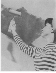
NEW PAINT ROLLER, shown in photograph, has a handle that holds the paint. Made of Bakelite polyethylene, the container-handle is squeezed as the roller is used, feeding paint to the roller through its perforated core. The new applicator is especially useful for coating ceilings since drip is eliminated. A pouring spout and protective cover for roller are included.
