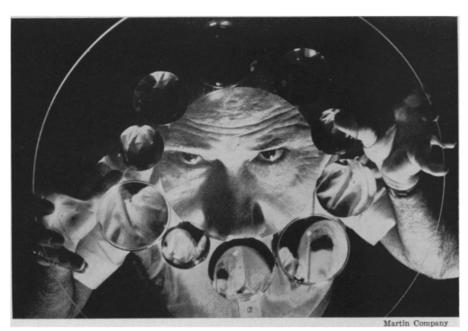
EYEING LASER LENSES—This Martin Company optical engineer who is peering at an array of precision lenses prepared for laser research, can grind lens surfaces so smooth that molecules on the surface of one lens join with molecules on the other upon contact, providing the strongest possible bond between them.
