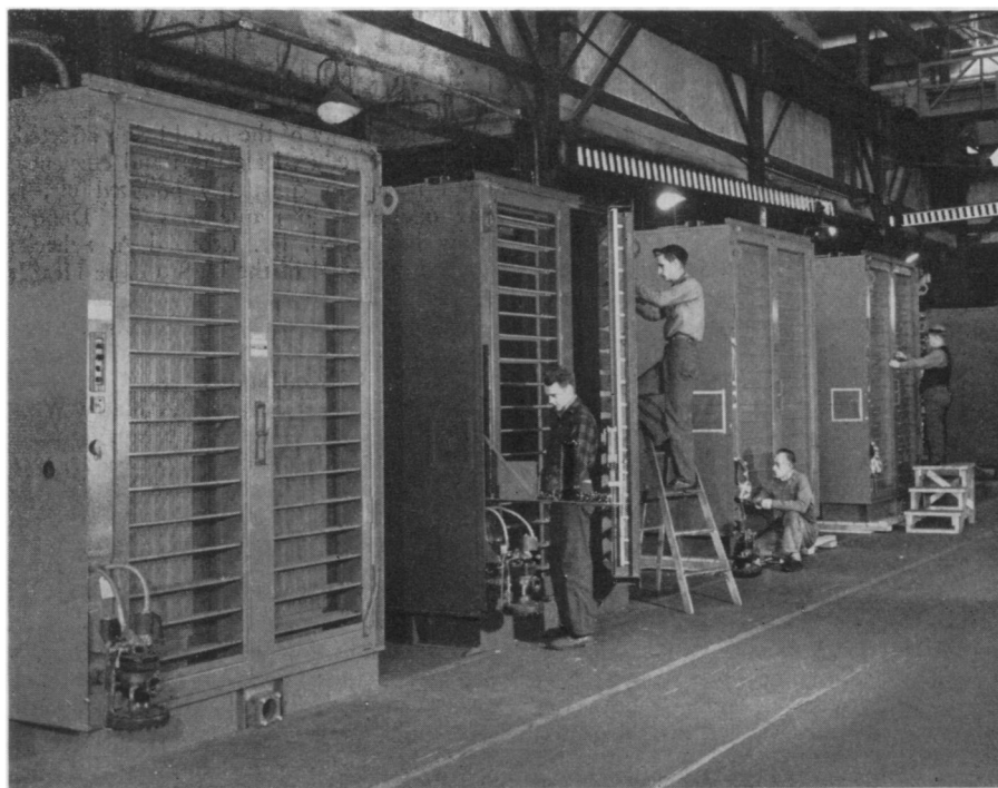
DUST VAULTS —Electronically-scrubbed air for steel mills is in the making on this assembly line at the Westinghouse Sturtevant Division plant in Hyde Park, Boston, Mass. The vault-like cubicles contain Precipitron cells, the electronic air cleaners which remove 90 percent of all air-borne dirt and dust. Each of these cubicles can clean more than 36 tons of air every hour.
