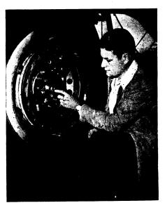
ANTI-SKID-DEVICE—The centers of all four main wheels of the Stratofreighter are equipped with this automatic device which sets braking action to prevent skids from any cause. It weighs only three and onehalf pounds.
