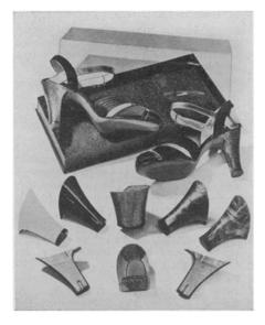
thermoplastic evenly distributed about a sixteenth of an inch thick and without seams. The plastic slightly impregnates the wooden core to form a permanent bond. Dull or shiny finishes in many colors are available.
