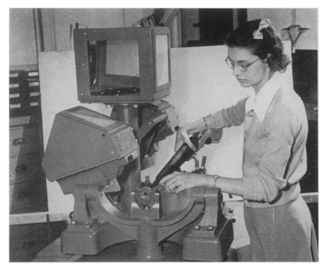
DONE WITH MIRRORS—With this optical sighting gage invented by General Electric engineers, the sights of a Garand rifle can be correctly adjusted in less than two minutes and without firing a shot. The job used to take up to 13 rounds of ammunition.
