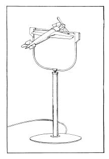
mitted through a cable, actuate the control surfaces of the model airplane shown in the lower cut. This model plane is so supported that it is free to turn in any direction. Wind from a fan blows against it so that it tilts or turns or noses up or down in response to the movements of the student aviator just as a real airplane would do under like circumstances. A patent has been awarded for this invention.
